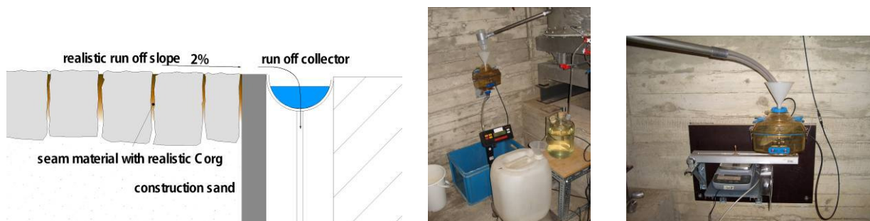
Figure 2. Collection and measurement of run-off and groundwater recharge.
